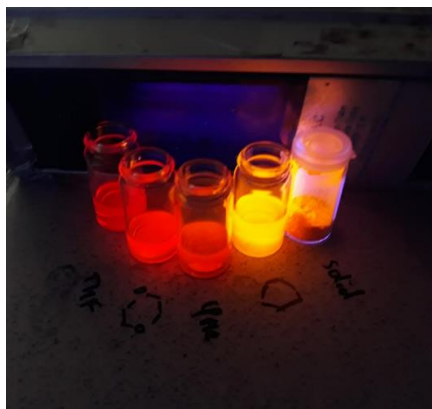
Figure: Solvatofluorochromism of TAPP obtained from 4-formyl-2,1,3-benzothiadiazole. Red emission in polar solvents is visible.
